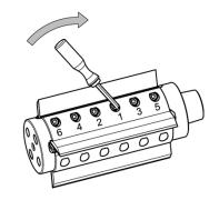
Clamping screws are loosened in the reverse order than when clamped. Undo the clamping screws in exactly the same order depicted in the graphic. First undo clamping screw (1) on all knives. Then undo clamping screw (2) and so forth on all knives.
