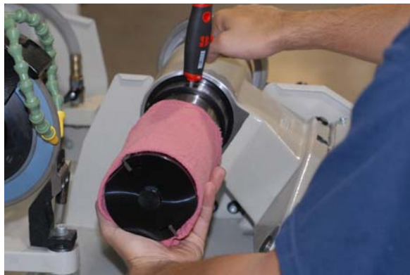
Use gloves or shop towels when mounting a Helicarb Tool
