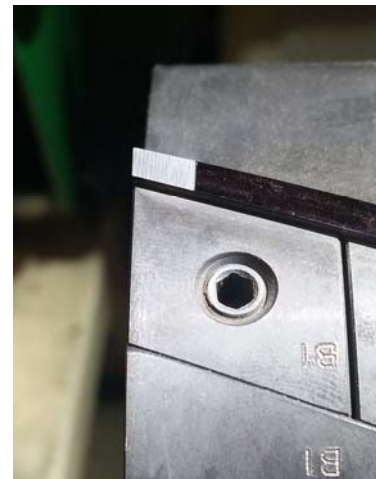
Use black marker to see effect of sharpening
